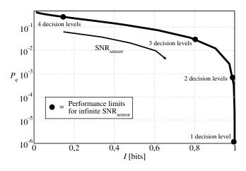
Fig. 4. Probability of decision error, as a function of the mutual information, in a scenario with uniform clustering and noisy communication links (p = 0.05). The limiting (SNR<sub>sensor</sub>  $\rightarrow \infty$ ) operational point with various number of decision levels are shown.
