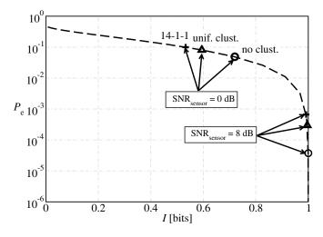
Fig. 2. Probability of decision error, as a function of the mutual information. The operational points for various clustering configurations and two sensor SNRs are shown.
