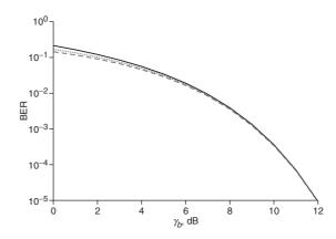
Fig. 1 Upper and lower bounds for BER of DQPSK transmission with Gray coding over AWGN channel
