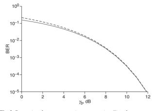
Fig. 2 Comparison between approximate expression (8) and exact expression for BER of DQPSK transmission with Gray coding over AWGN channel
