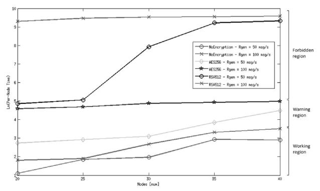
Figure 9. Logarithmic representation of the stream delay as a function of the number of nodes of the Graph, evaluated both without security mechanisms, as well as with cryptographic features.
