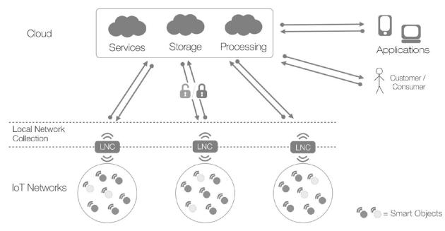
Figure 1. Different actors and layers involved in IoT scenarios: sensed data are sent from IoT networks to the Cloud, which provides services to consumers. At an intermediate level, preliminary local operations, such as data collection, processing, and distribution, may be carried out.
