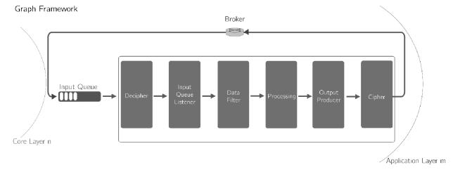
Figure 6. Detail of the structure of a single Graph node: the decryption module is activated when the node is a listener of a secured stream, while the encryption module is activated if the node generates a secured stream.
