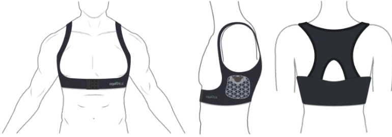
Figure 1.2 Equivital EQ02 LifeMonitor sensor belt positioning.
