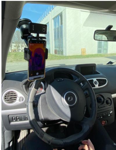
Figure 1.3 FLIR One Pro LT thermal camera positioning inside the vehicle.
